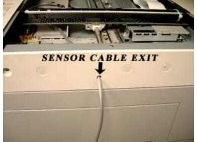
It just so happened there was already a hole in the Canon, but your copier may not have a hole available, so you may need to drill a ¼" hole in order to feed the sensor cable out of the scanner area. Here is a photo of a Samsung C8380ND where the application calls for a hole to be drilled. The hole is on the right side of the scanner unit.
